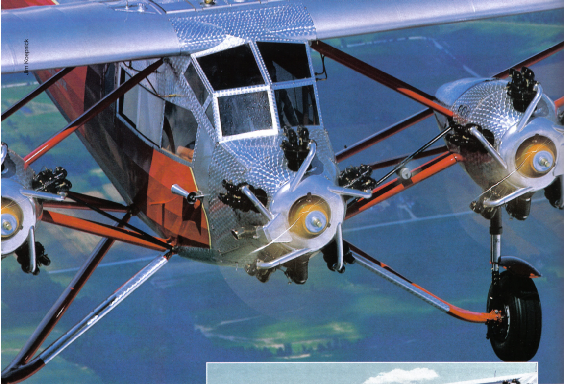
The three Kinner K-5s swing a trio of Sensenich fixed pitch, wood props to move the K-5 Air Coach along at a stately 100-110 mph. Al Ball of Santa Paula, CA gets all the credit for restoring the three Kinnners to outstanding condition.
