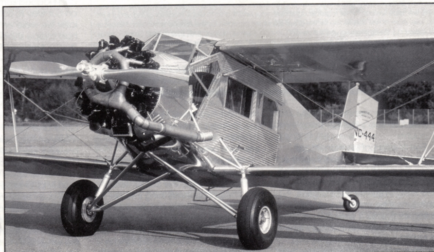
The PT-6F was advertised as an all-metal aircraft but, as can be seen, the craft was covered in fabric.
