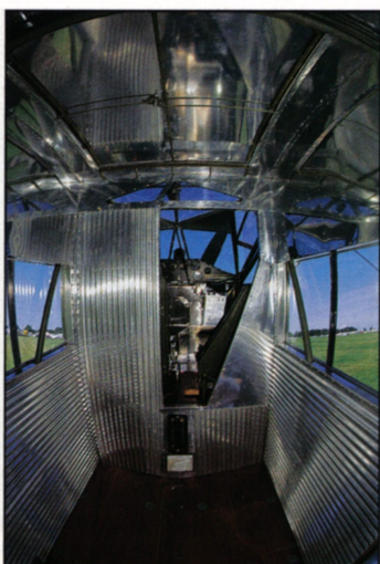
The cabin is lined with corrugated aluminum, and can hold up to 156 cu. ft. of cargo. The doorway at the front of the cabin is normally filled with a door, which is shown removed in this shot. It was one of just a very few items that had to be completely built from scratch during the restoration of the biplane.
