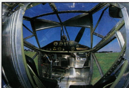
(Left and below) The cockpit is still just as it was while the Cunningham-Hall was working the bush in Alaska and the northwestern U.S., although it's probably a lot cleaner than those days! The only addition is a removable radio stack mounted on the right side, between the co-pilot's legs. The co-pilot's seat (inset) is a novel affair — it can be folded and then stowed below the cockpit floor, giving a few more crucial feet to the cargo compartment.
