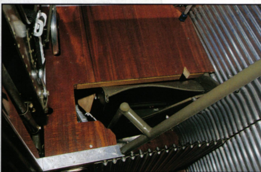
The cabin is lined with corrugated aluminum, and can hold up to 156 cu. ft. of cargo. The doorway at the front of the cabin is normally filled with a door, which is shown removed in this shot. It was one of just a very few items that had to be completely built from scratch during the restoration of the biplane.
