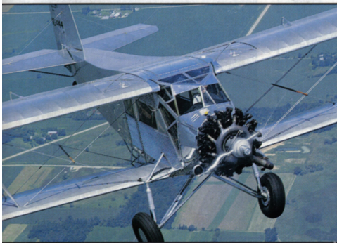
A 440 hp Wright R-975 currently powers the Cunningham-Hall, although a 450 hp Pratt & Whitney R-985 is in its future. The cockpit is elevated above the cargo compartment, and with all of the windows, it has excellent visibility in just about every direction.
