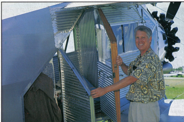
Greg Herrick shows off the dual cargo doors. The aft door can be removed by pulling a couple of pins linked with light chain, and if needed, even the forward door can be removed. If that won't work, then try this . . .
