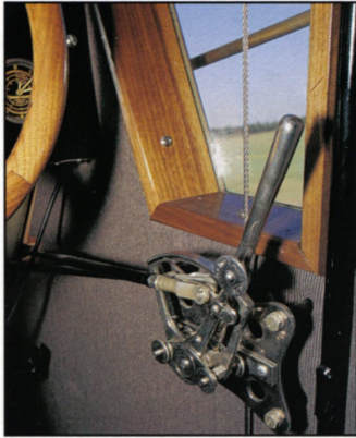
This nickel-plated throttle quadrant, one of two installed in the airplane by Air France when the Buhl was converted back to a Wright engine, has been maintained as part of the historical legacy of the "Packard Buhl."
