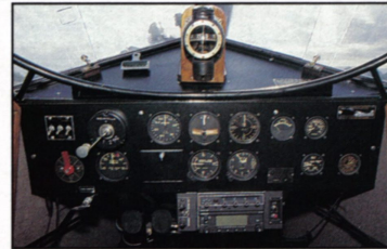
The instrument panel is just as it appeared over 60 years ago when the airplane was exported to Argentina after serving as one of the Packard diesel engine demonstrators in 1930. The Star Pathfinder compass is there, along with a Bulldog clip for holding a map. Both front windows can slide open after unscrewing the small clamps. They must let in a tremendous amount of air!
