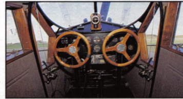
This wide shot of the cockpit shows the dual control wheels, along with the steel tube interior bracing. There are three of those "hoops" visible in the interior of the Airedan, adding to the strong nature of the cabin.
